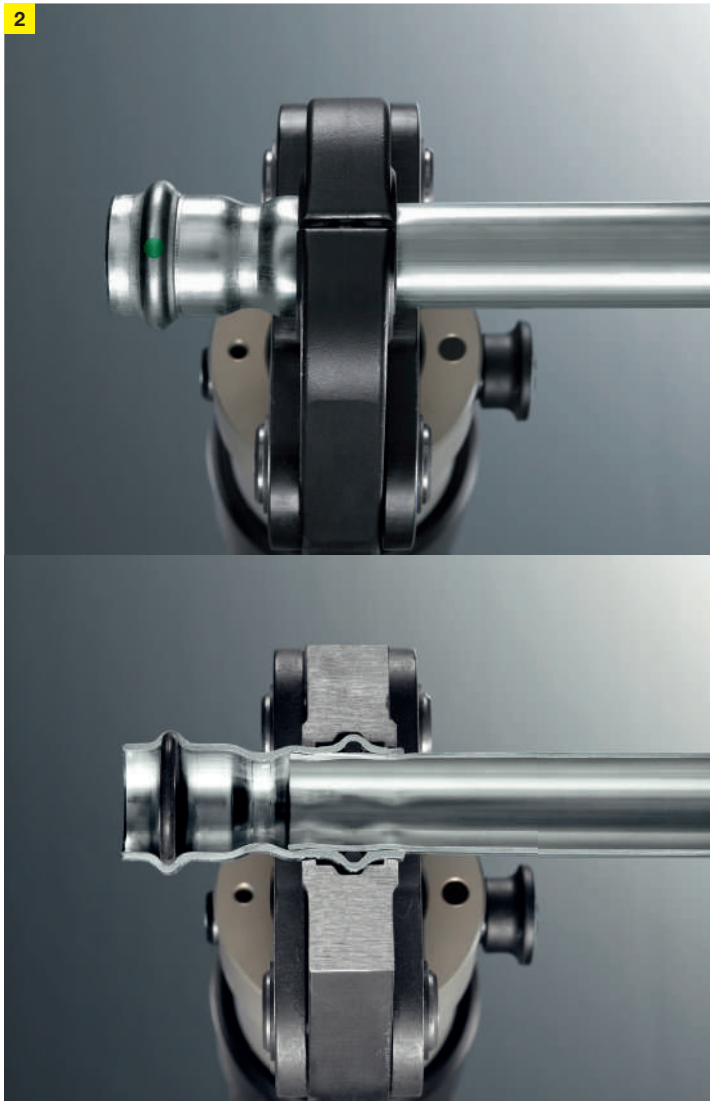
The Viega SC-Contur can be clearly recognised by a coloured marking on the bend. Inadvertently unpressed connectors are recognised as leaky by a central leakage test.
