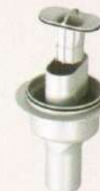
4982.94 Vertical model drain for installation heights from 40 mm, drainage capacity: 1.05–1.1 l/s, water head seal: 50 mm (fire protection pipe lead-in possible)
