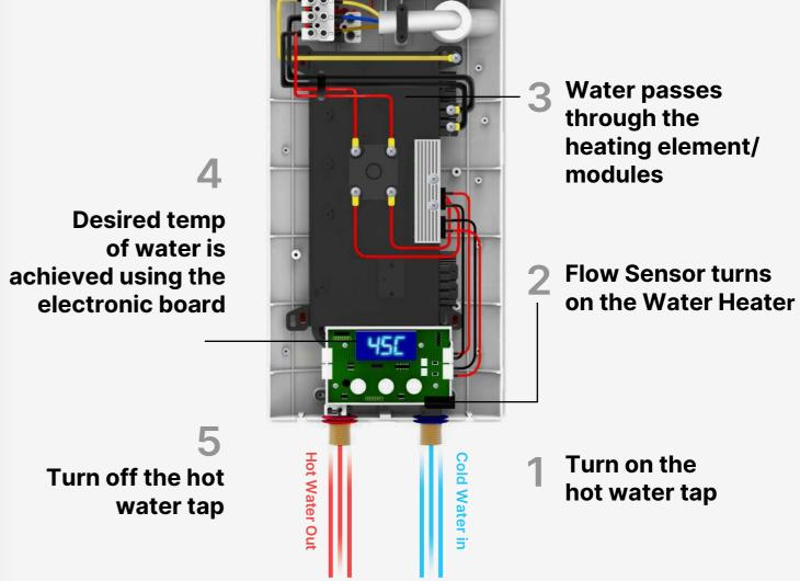
Appliance turns off as soon as the tap is turned off. No power is consumed until the hot water tap is turned back on
